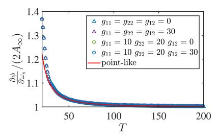
FIG. 6. Phase gradient as a function of the interrogation time T. The estimate based on a point-like particle subject to the centripetal force agrees well with numerical calculations and is largely independent from the presence or absence of interactions.
